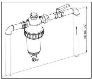
Fig. 1: In-Line installation
