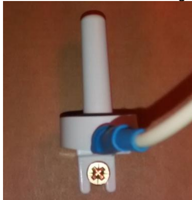
Solar Panel sensor mounting
